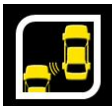
Fig 4: When BSD Region of Interest is Occupied (Vehicle Detected)
