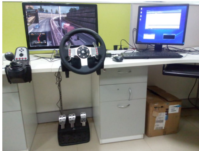
Fig.6: Snapshot of Verification System Set-up
