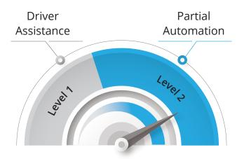
In the current market, most vehicles are already equipped with Level 1 (Driver Assistance) and Level 2 (Partial Automation) automation or Advanced Driver Assistance System (ADAS) features that include lane-keeping assistance, emergency braking assistance, proximity warning, adaptive cruise control, and so on. Moreover, in various countries, the installation of the ADAS system has become a regulatory requirement in all upcoming vehicles.
